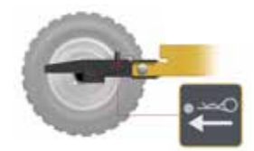
Secure the lock using a split pin
