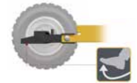
Move the lever arm up using your foot
